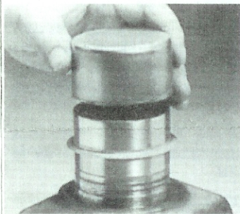
6. Place installation tool over sleeve.
