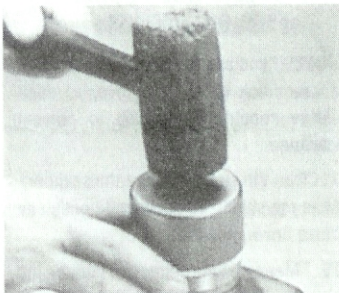
7. Tap tool to install sleeve over shaft.
